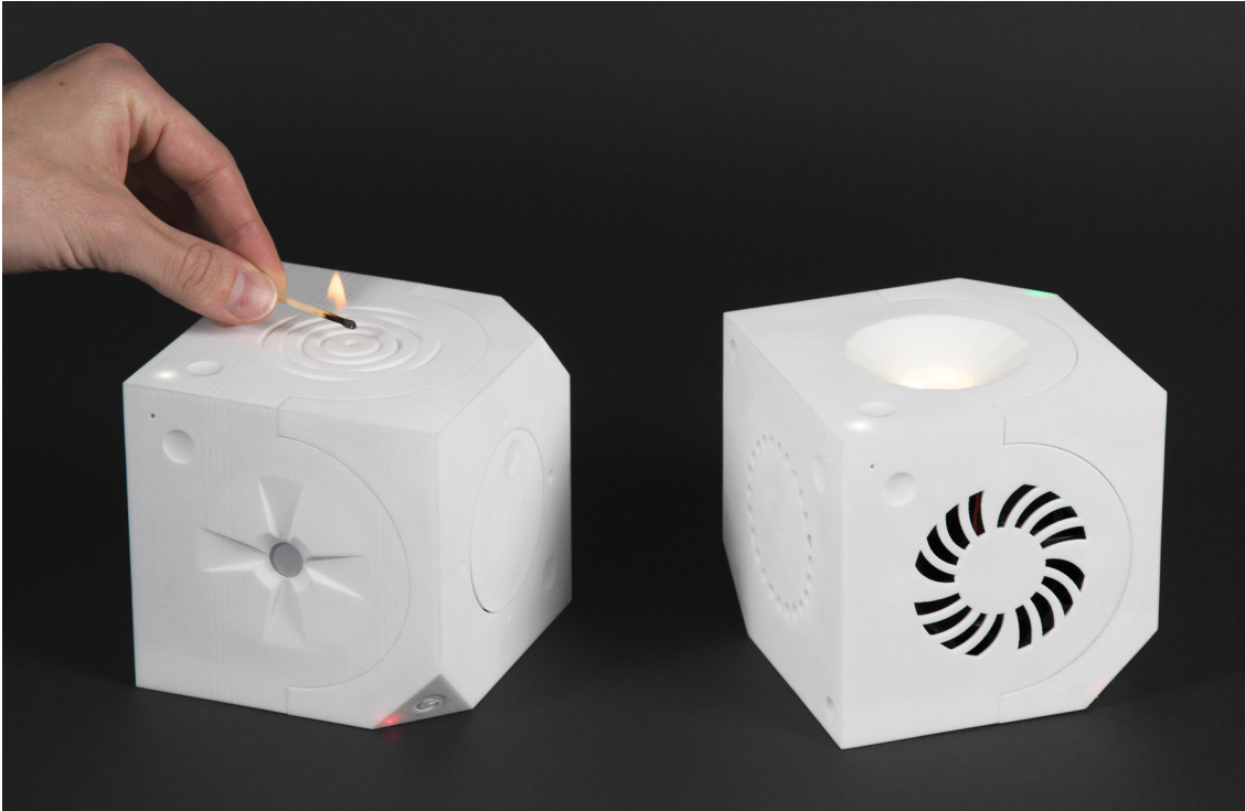
Figure 3: The Loaded Dice sense heat and transmits it as light.
